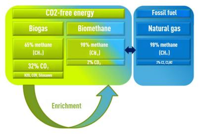
SUEZ AIR & CLIMATE has extensive experience in biogas treatment and collaborates with Prodeval and uses the VALOPUR® **membrane upgrading** system to produce high-purity biomethane.
