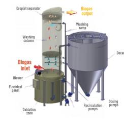
The stream coming from the Decanter **Second** stage reaches decanter, where the elemental sulfur S<sup>0</sup> decants. This by-product can be directed to a leachate plant, managed externally (as it is not hazardous) or used for manufacture of phytosanitary products.
