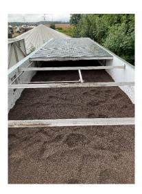
Additionally, it is worth noting that advanced biofilters do not require chemicals, control instruments, or recirculation or dosing pumps, enabling **simple and cost-effective control systems**. Furthermore, the process effluents are not considered toxic or special, allowing for easy management.
