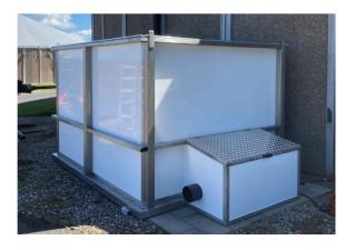
The Biocassete is made of a fibreglass sandwich panel with polyurethane foam insulation inside. The contaminated air is introduced at the bottom of the system and by means of an upward flow is purified through the filter medium. The biomedia is humidified with sprinklers located on its surface, using mains water connected to the bottom of the equipment.
