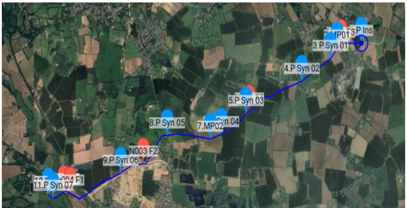
Overview of the pipeline showing the incidents detected during the inspection, synchronizer locations (P SYN), insertion point (P INS), and extraction point (P EXT).
